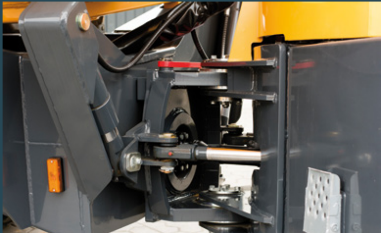
Articulated swivel joint with stabilization cylinder.
